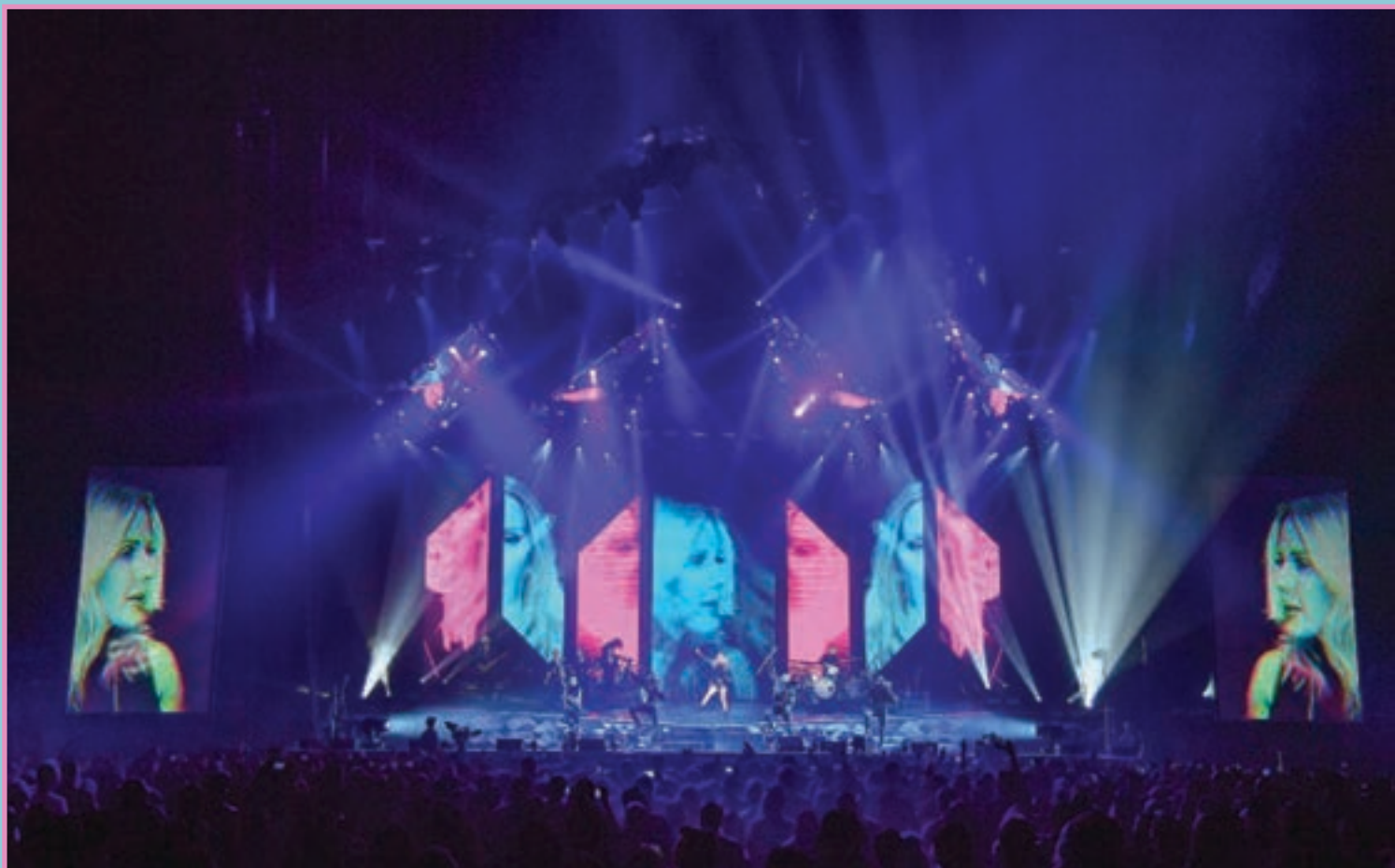
The LED in the center receives content via a d3 Technologies media server; it's flanked by two screens fed by two Barco HDXW-20 projectors.
