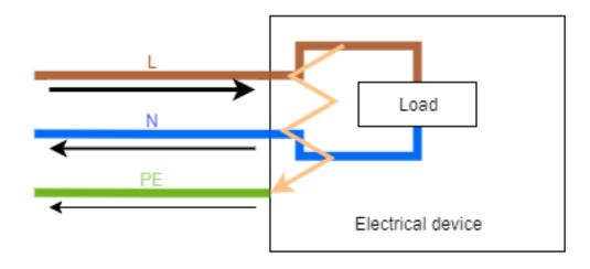
RFI filters: Radio-frequency interference filters are connected to the mains and filter current to reduced harmonics in the power supply or generated by the electrical device. To suppress those harmonics an RFI filter outputs the filtered current to the earth. Because an RFI filter contains capacitors, it will produce a current spike at power-up.
