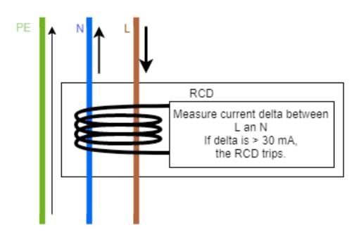
It is required in every electrical installation. The main specifications for an RCB are:
