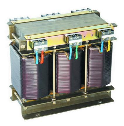
An isolation transformer contains 3 primary coils and 3 secondary coils. Each primary coil transmits the magnetic field to its secondary thus providing power to the secondary output. The neutral is generated by connecting one of each end of the secondary coils.
