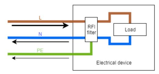
**Variable Frequency Drive (VFD)** require such RFI filters to comply to the EMC directive. The EMC directive specifies limits for the radio interferences generated by any electrical appliance. As a consequence, the manufacturer integrates an RFI filter in every VFD.
